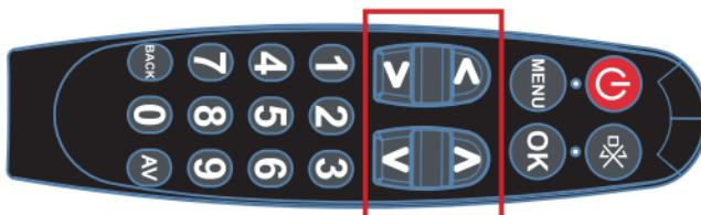
To activate this mode, press and release the [MENU] button until the LED indicator light comes on. You can now use the **UP/DOWN/LEFT/RIGHT** navigation buttons.
